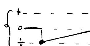
Shows the movement of the pitch bender (on the left hand side of the keyboard). The players should play the pitches indicated on the (normal) note system with his right hand, while moving the bender as indicated by the graphic with the left hand. The resulting effect should be the one notated on the third ('effect')-line (above the two 'normal' ones).
